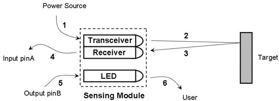
Figure 7. A design of the sensing module
