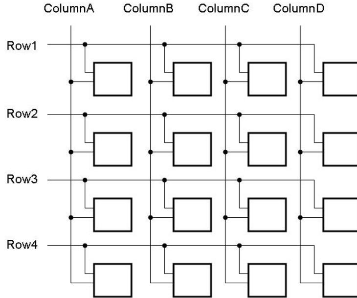
Figure 11. The Row Column Scanning technique
