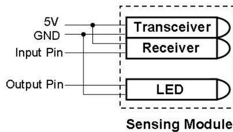
Figure 10. The circuit of sensing module
