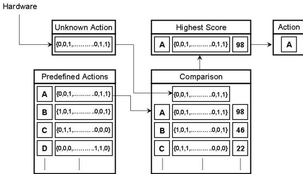
Figure 15. The detail data flow of PM approach
