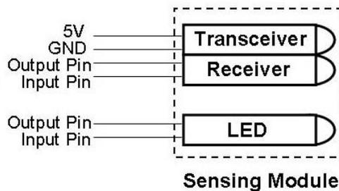
Figure 12. A modified circuit of sensing module
