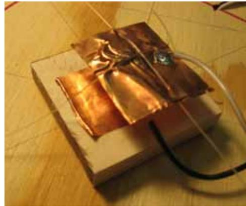
**Figure 8: The pressure sensor**
